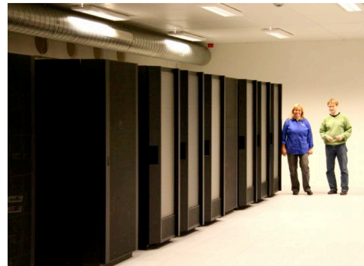
Elster and Linid behind Njord, NTNU's new 7.5 TFlops IBM Power System P5+ Supercomputer
