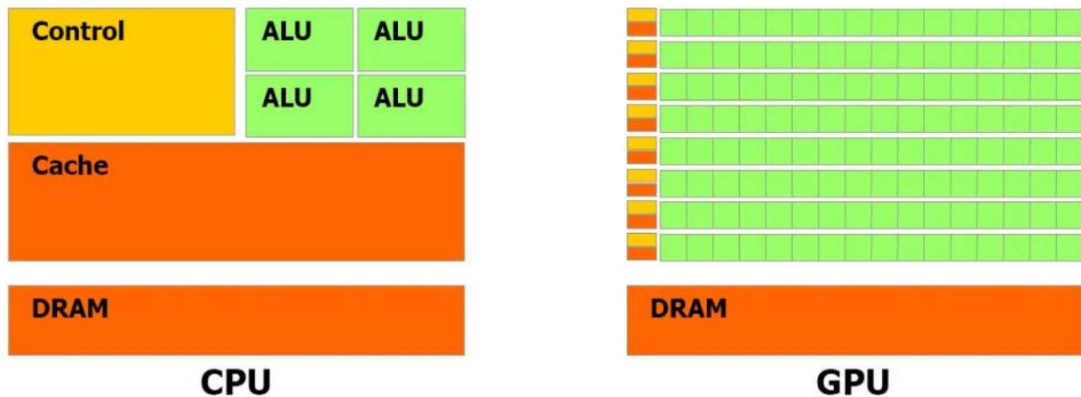
Figure 4: Transistors used for data processing for the CPU and GPU. Figure is from [8].
