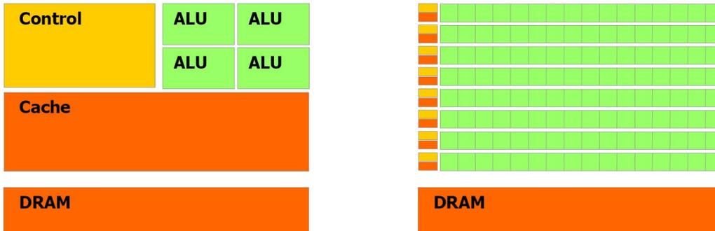
Figure 2.2: Transistors dedicated for data processing: CPU vs. GPU. Figure is taken with permission from [12].
