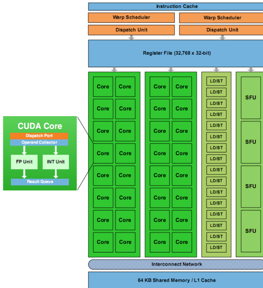
Figure 2.5: Fermi streaming multiprocessor, taken from [5] with permission from NVIDIA.
